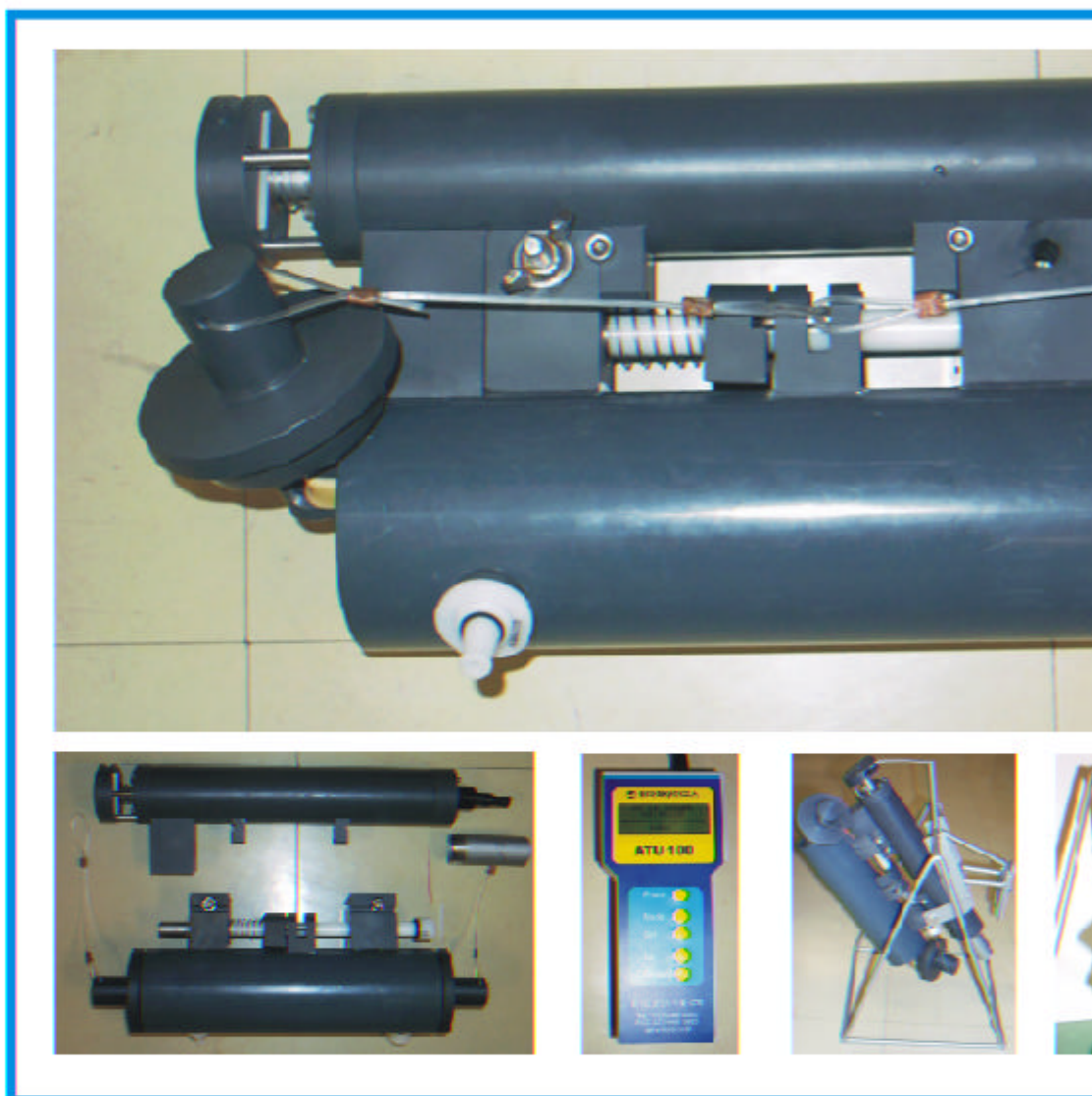
➤ Assembled AUTTLE for automatic operation (upper), detached control panel and time setting unit (ATU-100), and sampling procedures (lower)
